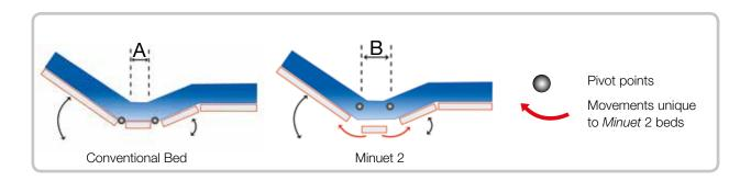
Compared to a conventional profiling bed (A), the *Pro-Contour Advance Profiling* on the four-section *Minuet 2* beds raises the pivot point of the backrest and thigh section closer to the client's natural pivot point (their hip joint) (B). As a client moves from a lying to a more upright position, this reduces abdominal compression, and improves comfort.
